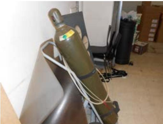
19. Nitrogen gas cylinder in Microlux Technology.
