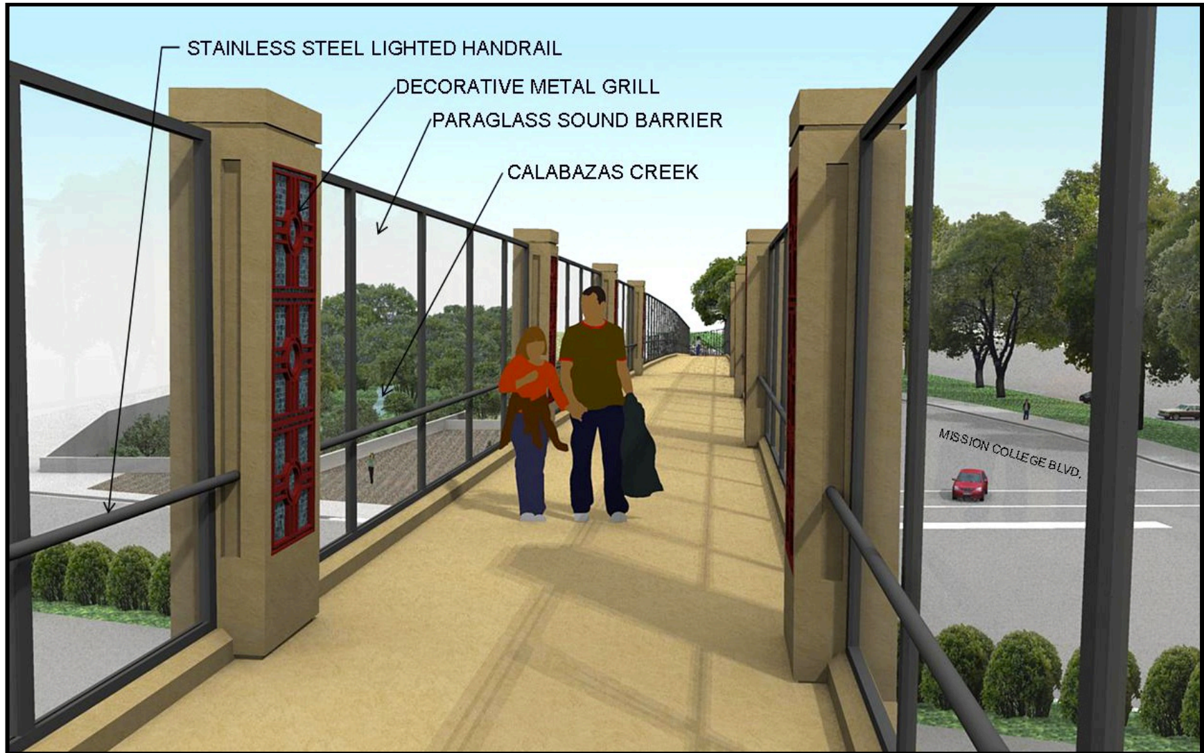
Illustration 3 – View from the Bridge Deck on the Highway 101 Pedestrian Overcrossing
