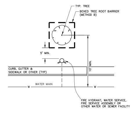
METHOD A: LINEAR TREE ROOT BARRIER MUST BE LOCATED 5' MIN FROM NEAREST WATER APPURTENANCE. BARRIER MUST EXTEND PAST TREE DRIP LINE OR 10' MINIMUM, WHICHEVER IS GREATER.
