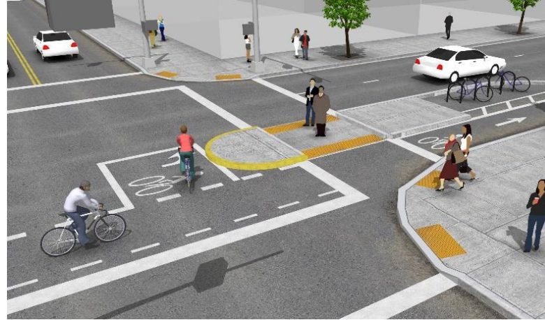
Median Refuge Island
