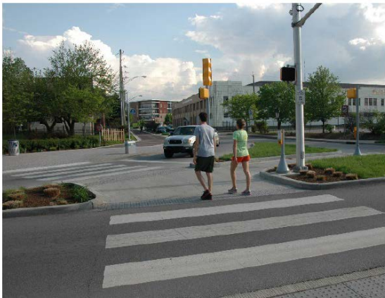
Improved Right-Turn Slip Lane Design
