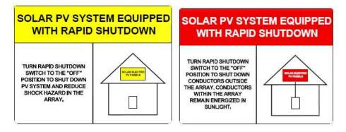
Informational note: ANSI Z535.4 provides guidelines for the design of safety signs and labels for application to products. A phenolicplaque with contrasting colors between the text and background would meet the intent of the code for permanency. No type size is specified, but 20 point (3/8") should be considered the minimum. CEC 705.12 requires a permanent plaque or directory denoting all electric power sources on or in the premises.
