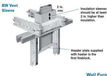
Cut out the drywall above the furnace so the header plate that connects the flue to the top of the furnace can be inspected. The drywall can be held in place with screws and removed when the inspector arrives
