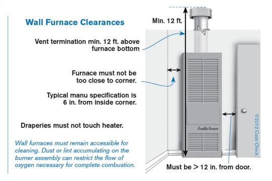
Wall furnace vents must extend at least 12 ft. above the floor. For apartments on the top story, this will require vents extending higher than those from lower floors.
