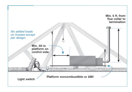
Access opening, minimum 30" X 30" (exc. –may be 22" X 30", provided largest piece of equipment can be removed) must be located within 20' of furnace
