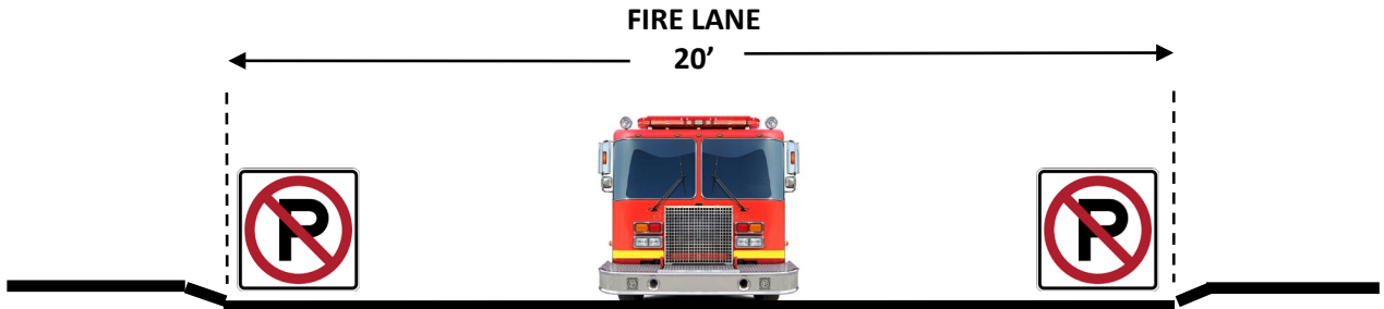
FIGURE 1 – Engine Road Width
