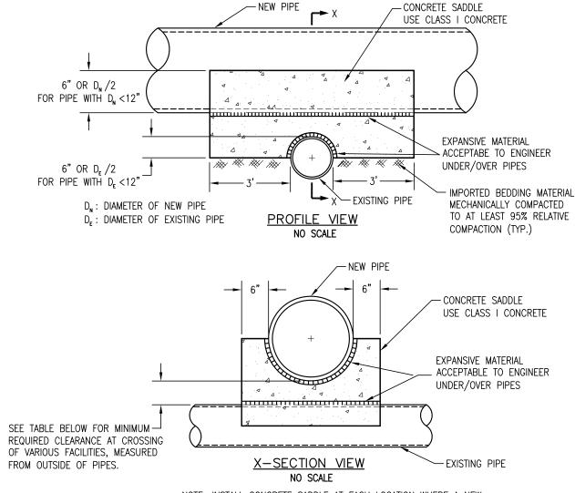
NOTE: INSTALL CONCRETE SADDLE AT EACH LOCATION WHERE A NEW UTILITY CROSSES AN EXISTING UTILITY WITH LESS THAN 12" CLEARANCE.
